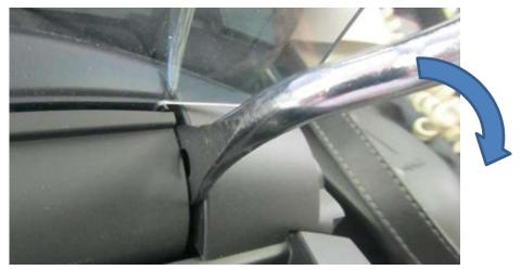
Note: Adjust force applied to the tool by carefully watching the clearance..
