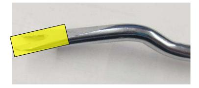
5. Insert the tool in the clearance then push the ADD combiner assembly to left by using the tool as leverage.
