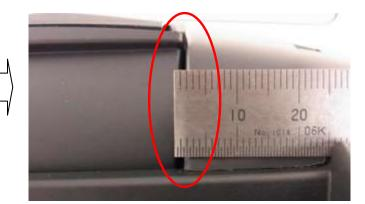
3. To establish the clearance, hold the edge of the ADD combiner and push it to left lightly.
