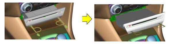
3) Push the fastener areas to release the SST out of the fastener.
