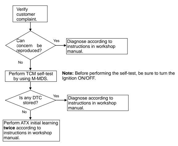
XThe initial learning forcibly actuates each valve in the valve body and verifies their operation. During this operation, ATF is circulated through the valve body having a flushing effect.
