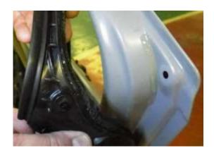
9. Install the weatherstrip to the door panel and press the bonding area of it.
