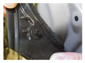
5. Clean the bonded area of weatherstrip and door panel. (Dotted line area of picture)
