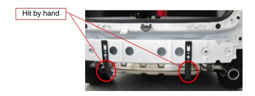
3. Remove the stay fixing bolts, then remove the bumper stays (both sides).
