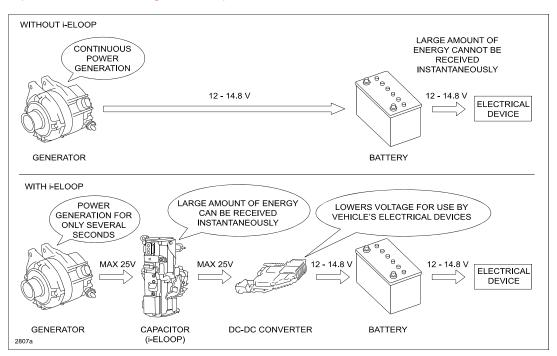
NOTE: The capacitor stocked as a repair part must be used within 2 years after production date. The production date is indicated on the outer case of the repair part. When the capacitor is stored, keep it upright. When you dispose of the vehicle or the capacitor, be sure to conduct the forced discharge of the capacitor before disposal according to MS3 on line or Workshop Manual (section 13-17 CAPACITOR (i-ELOOP) COMPULSORY DISCHARGE [i-ELOOP]).
