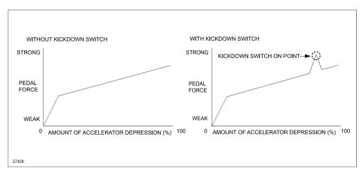
The driver can control the kickdown by knowing the amount of accelerator depression. The kickdown switch is only a measure of the kickdown. An electrical signal is **not transmitted** by the kickdown switch turning on/off, and vehicle control is not affected.
