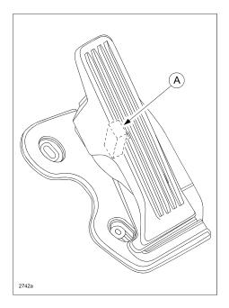
A kickdown switch (A) has been adopted to determine that the customer has fully depressed the throttle pedal for maximum acceleration. A load can be felt while the accelerator pedal is being depressed and when it is further depressed the kickdown switch is activated. A click is felt when the kickdown switch is activated.
