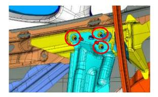
(2) Place the two brackets (upper and lower) in the back of the reinforcement and pass the stud bolts through the holes in the reinforcement.
