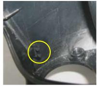
2. From the inside of the power outer mirror, remove the two tabs shown in figure using a tape-wrapped flathead screwdriver.
