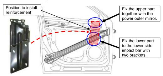
(1) While holding the power outer mirror, place the reinforcement either by passing three stud bolts of the power outer mirror through the holes in the reinforcement and tighten with three nuts or by aligning three tap holes of the power outer mirror with the holes in the reinforcement and tighten with three bolts (depending on mirror design).
