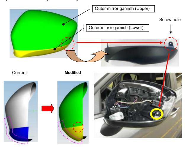
**Note:** The modified outer mirror garnish is provided without paint and consists of two parts (upper and lower).
