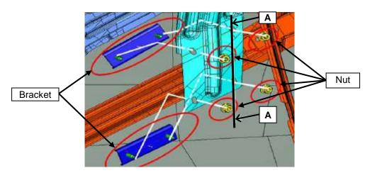
(3) Tighten with 4 nuts to fix the reinforcement onto the side impact bar-lower.
