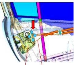
Door lock knob cable Rear door latch and lock actuator
