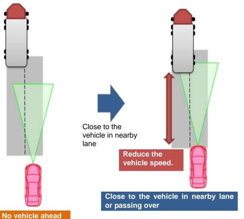
2. On a winding road, the vehicle in nearby lane is entering the radar sensing area. (Change from constant speed mode to headway control mode and speed reduction.)
