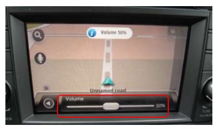
2. While voice guidance is active and volume bar is shown, turn the volume button. Then, actual Navigation voice volume is shown at right side of the screen.
