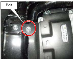
4. Remove the nut from the PCM bracket.
