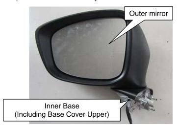
9. Install the inner base to the outer mirror using new screws (included in the base cover set).
