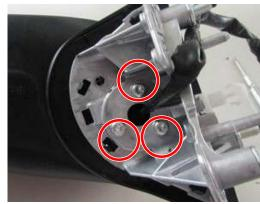
10. Push through the wire harness and install the new push nut (included in the base cover set) as per below picture.
