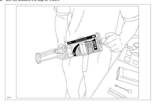
8. Begin squeezing the applicator gun trigger until clear dampening material starts to come out of one side.
