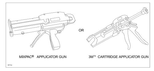
**NOTE:** Either applicator gun can be used, however, the 3M cartridge applicator gun is normally less expensive than the Mixpac applicator gun.
