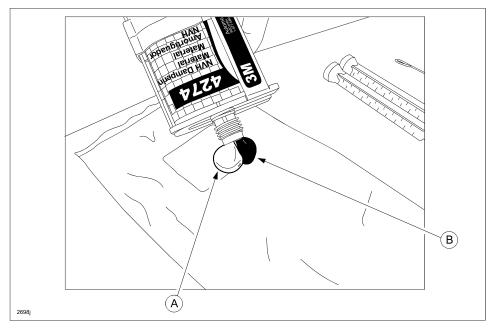
10. Insert the mixing nozzle onto the tip of the dampening material, then screw in the removed cap and tighten.
