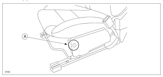
b. Pull up the front of the side cover to disconnect from the hook (A). This allows for working space between the seat cushion (B).
