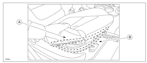
To eliminate this concern, three (3) clips (per seat) have been installed on the seat frame to increase the grasping force of the folding collars.
