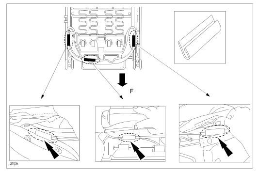
**NOTE:** DO NOT INSTALL THE CLIPS BACKWARDS. If the clips are installed backwards, they will be ineffective and will not reduce the clearance in the seat pan. In addition, if the seat cover comes loose again, the clips may completely fall off the seat pan.
