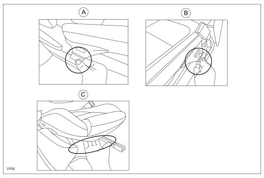
d. Install the three (3) clips on the seat frame flange (front passenger seat shown below).
