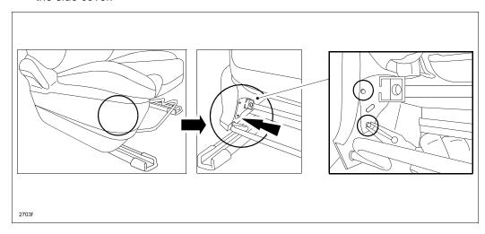
b. Pull up the front of the side cover to disconnect it from the hook (A). This allows for working space between the seat cushion (B).
