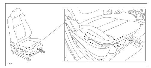
The front seat cushions are attached to the seat frame (B) using folding collars (A). These collars may become loose and slip off the seat frame when force is applied (i.e. customer entry) to the side of the seat cushion.
