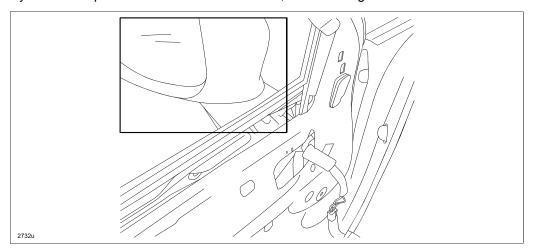
12. While holding the power door mirror, place the reinforcement passing three (3) stud bolts of the power door mirror through the holes in the reinforcement and tighten the three (3) nuts.
