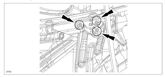
13. Place the two (2) brackets (A) (upper and lower) in the back of the reinforcement and pass the stud bolts through the holes in the reinforcement.
