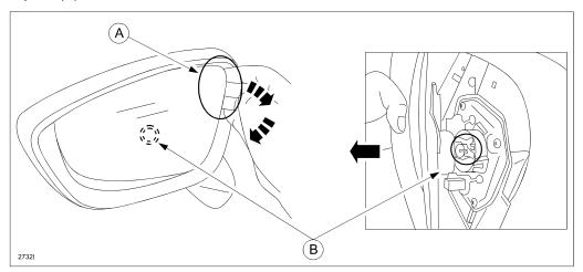
5. Move the mirror glass left and right and up and down to make a space for your fingers to insert in the back of mirror glass. Press the mirror glass with your fingers toward you to disconnect the joint for adjustment gears (A) and (B).
