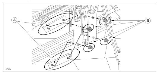
14. Tighten the four (4) nuts (B) to secure the reinforcement onto the side impact bar-lower. **Tightening Torque: 15 ft. lbf. {2.1 kgf-m, 20 Nm}**
