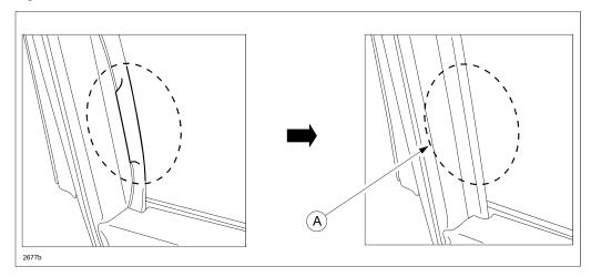
3. Degrease the area along location (A) of the door sash (B) and inside the glass run channel (C) as shown below.
