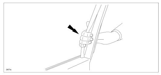
To prevent the glass run channel from slipping from out of position, a coating has been applied to the outer surface of the glass run channel to decrease frictional resistance.
