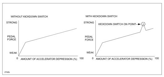
The driver can control the kickdown by knowing the amount of accelerator depression. The kickdown switch is only a measure of the kickdown. An electrical signal is <u>not transmitted</u> by the kickdown switch turning on/off, and vehicle control is not affected.
