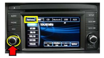
3. 1) Press and hold the audio power button.2) Additionally press "SEEK >>I"
