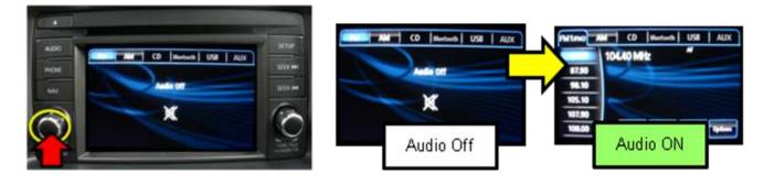
2. Change to FM mode by pushing the Power/Volume Dial, which is located in the left bottom.
