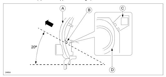
**NOTE:** If it is difficult to remove the center panel unit by hand, use a tape-wrapped fiber stick (B) or equivalent as shown below.
