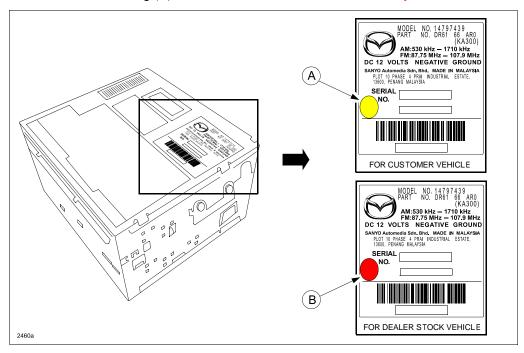
**CAUTION:**DO NOT INSTALL AN AUDIO UNIT WITH A <u>YELLOW</u> MARKING (A) ON LABEL ON A <u>DEALER</u> <u>STOCK</u> VEHICLE.
