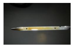
Your RX8 rotary engine will consume oil during normal operation. After 1,000 kms the dipstick should show about 30% - 50% less oil in the reservoir.
