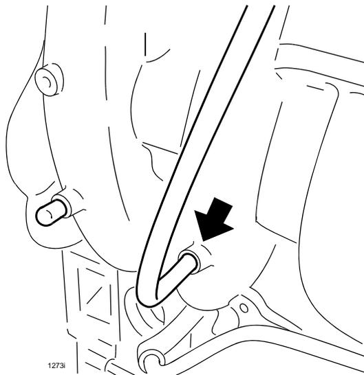
2. Attach vacuum hose of Manifold Vacuum Tester to intake manifold nipple.
