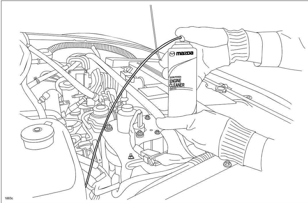
8. Have an assistant crank the engine. While cranking the engine, simultaneously depress the spray nozzle of the engine cleaner for a duration of 10 seconds. After 10 seconds, stop spraying and cranking at the same time. DO NOT depress accelerator pedal while cranking.
