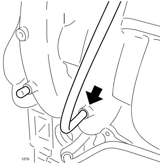
3. Disconnect vehicle barometric pressure sensor connector.
