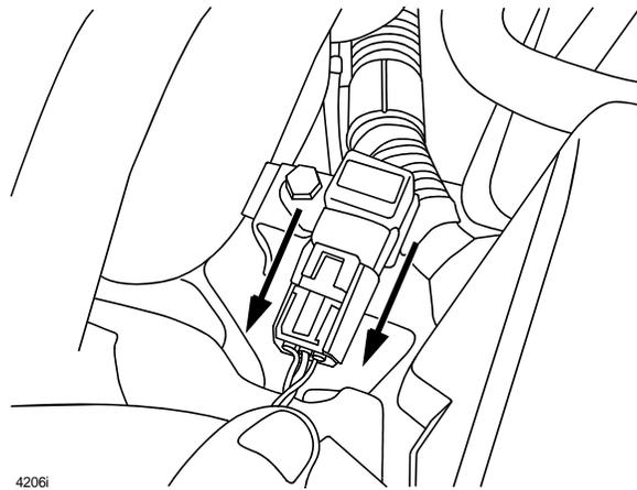
4. Connect SST to vehicle barometric pressure sensor and barometric pressure sensor connector.
