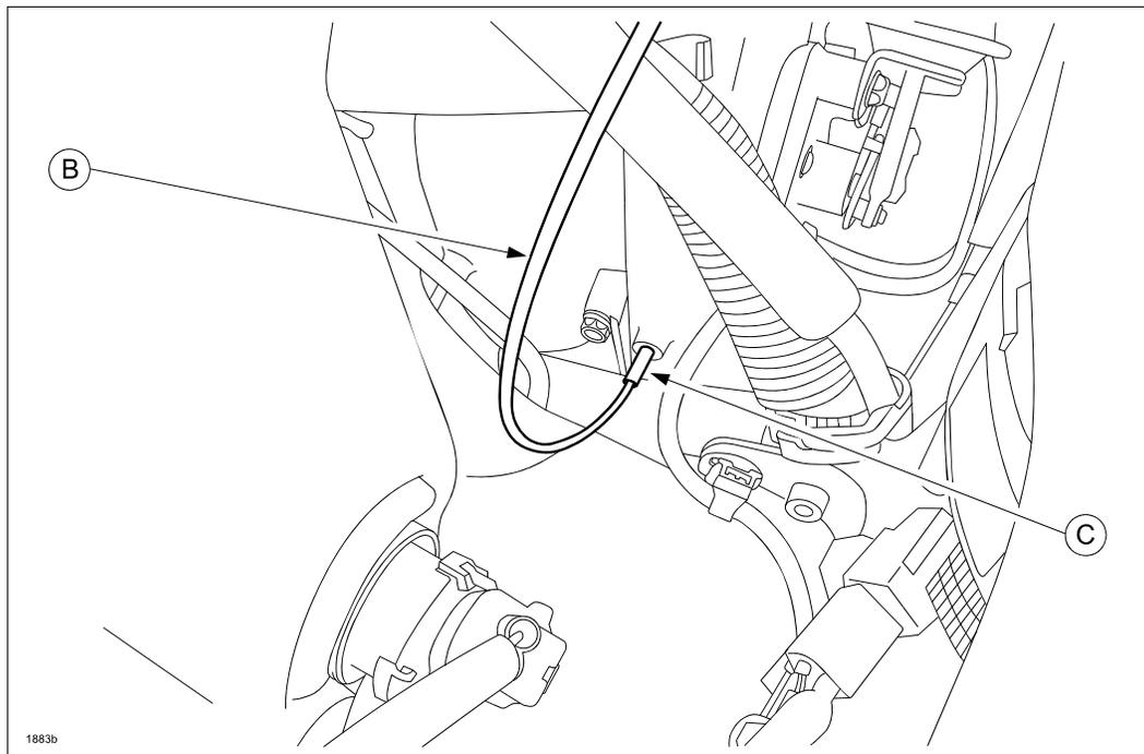
7. Attach engine cleaner spray hose to engine cleaner spray can nozzle.
