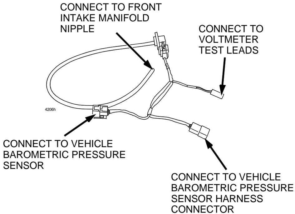
1. Remove the front vacuum plug or vacuum hose from the passenger side of the lower intake manifold.
