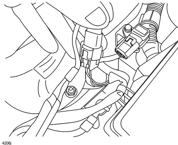
5. Connect positive lead of FLUKE meter to red wire of SST, and negative lead of FLUKE meter to black / green wire of SST.
