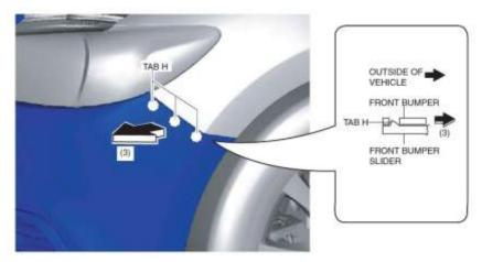
If you pull the edge of the front bumper to outside of vehicle before grommet removal, the fastening part of front bumper could be broken.
