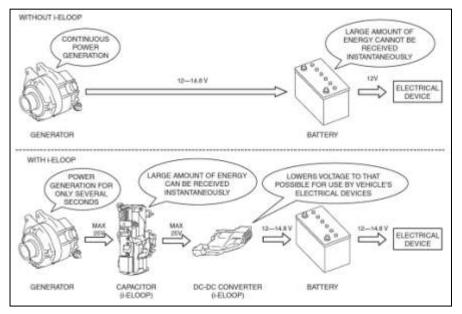
**Note:** The capacitor stocked as a repair part must be used within 2 years after production date. Production date is indicated on the outer case of the repair part.
