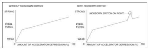
The driver can control the kickdown by knowing the amount of accelerator depression. The kickdown switch is only a measure of the kickdown. An electrical signal is not transmitted by the kickdown switch turning on/off, and vehicle control is not affected. 10. Front bumper removal (For previous steps refer to workshop manual [FRONT BUMPER REMOVAL/INSTALLATION]
