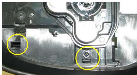
3. Pull to remove the outer mirror garnish (lower).
