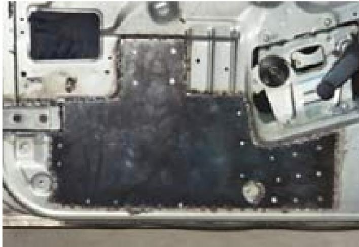
He made a template out of cardboard and transferred the shape to the metal plate. He used a plasma cutter and a grinder to shape the metal. He then used tack welds spaced about an inch apart to secure the metal plate to the inner door frame. (He also used self-tapping sheet metal screws to temporarily hold the plate tightly against the door frame while he welded it.)
