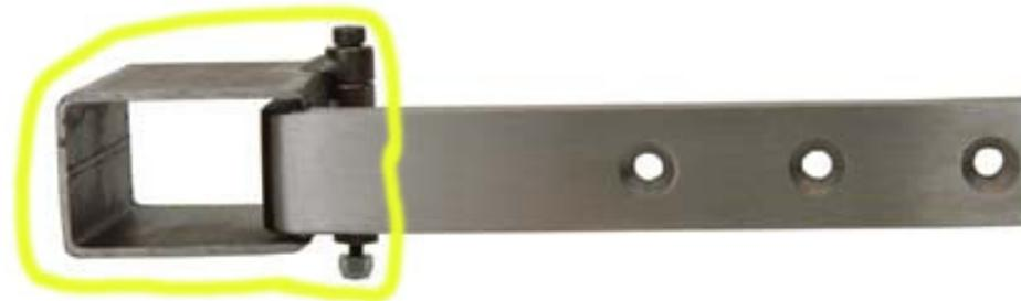
The hinge pockets are the rectangular pieces of metal that the hinge's arm rotates back into when the door is shut. I've circled the hinge pocket in the picture above. Above, the hinge arm is extended 90 degrees. The position of the hinge above is the position it will be in when your suicide door is open 90 degrees (straight out from the vehicle).
