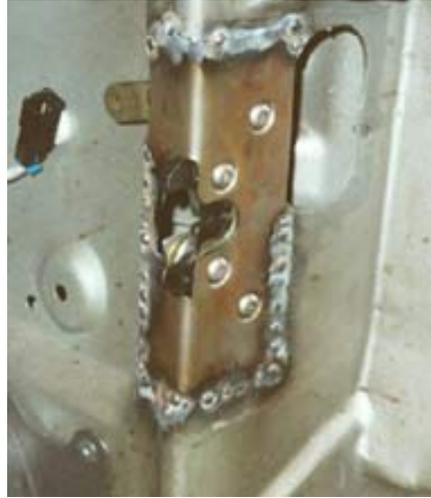
Now you need to install the strike pin and plate. To get it lined up perfectly, go ahead and latch the strike pin into the teeth of the latch that you just mounted. Then climb into the vehicle and pull the door together. Mark the position on the door jamb where the center of the strike pin needs to be positioned.
