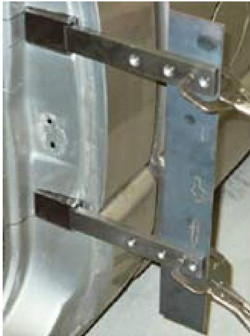
Remove the hinge arms and pull the the hinge pockets out of the holes. You now need to strip the paint from the openings prior to welding. Jason recommends using airplane strength paint remover. Just be careful not to get it on any other part of your car! Mask off all surrounding areas before using the paint remover. Otherwise you may end up ruining your paint job.
