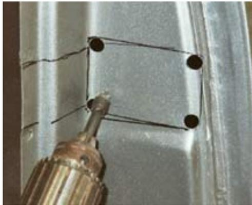
Then you can use a grinder with a cut off wheel to finish the job:
