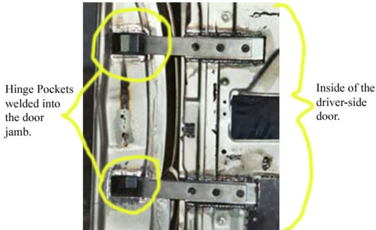
Now that you can clearly see how the hinges will be installed, you can begin mounting the hinge pockets. To choose the best location for each hinge pocket, remember these tips:
